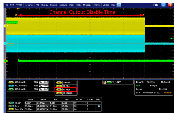
Figure 5-15. Channel Disable Setting Time
