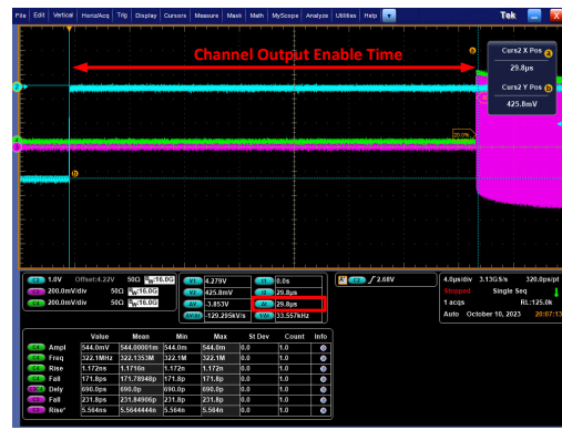
Figure 5-19. Channel Enable Setting Time
