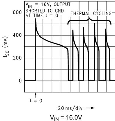
Figure 5-33. Short-Circuit Current vs Time (Legacy Chip)
