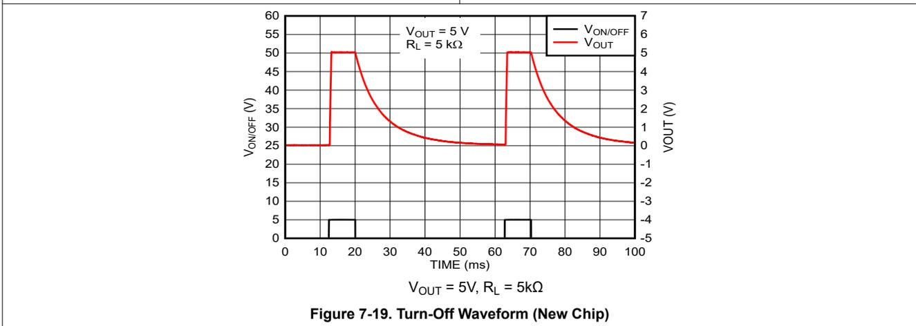
**Figure 7-19. Turn-Off Waveform (New Chip)**
