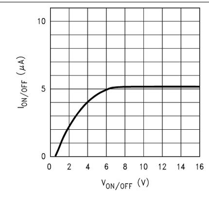
**Figure 5-54. ON/OFF Pin Current vs  $V_{ON/OFF}$  (Legacy Chip)**
