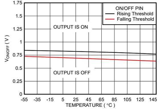
Figure 5-58.  $\text{ON}/\overline{\text{OFF}}$  Threshold vs Temperature (New Chip)
