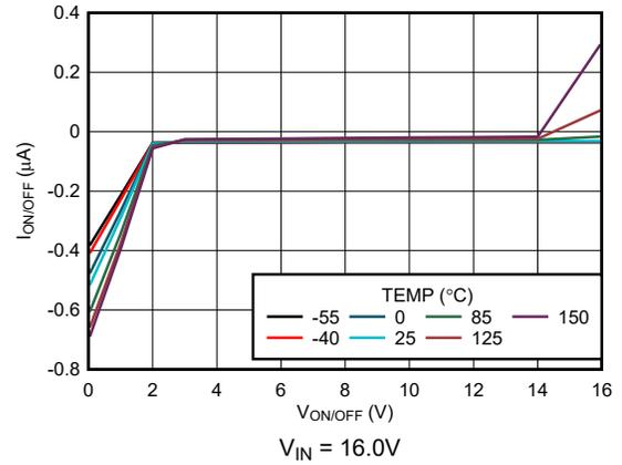
Figure 5-56.  $\text{ON}/\overline{\text{OFF}}$  Pin Current vs  $V_{\text{ON}/\overline{\text{OFF}}}$  (New Chip)
