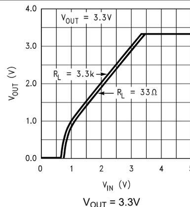
Figure 5-6. Output Voltage vs  $V_{IN}$  (Legacy Chip)
