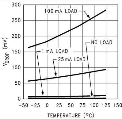
Figure 5-11. Dropout Voltage ( $V_{DO}$ ) vs Temperature (Legacy Chip)
