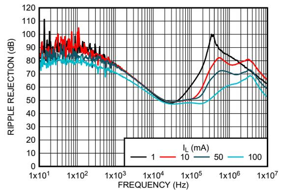
**Figure 5-42. Ripple Rejection vs Load Current ( $I_L$ ) and Frequency (New Chip)**
