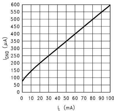
Figure 5-17. Ground Pin Current ( $I_{GND}$ ) vs Load Current (Legacy Chip)
