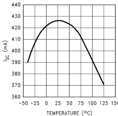
Figure 5-35. Instantaneous Short-Circuit Current vs Temperature (Legacy Chip)
