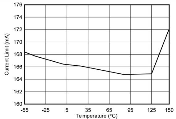
Figure 5-36. Instantaneous Short-Circuit Current vs Temperature (New Chip)
