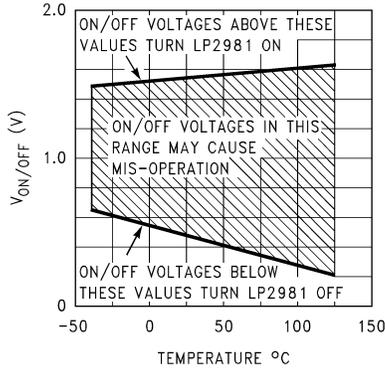
Figure 5-57.  $\text{ON}/\overline{\text{OFF}}$  Threshold vs Temperature (Legacy Chip)
