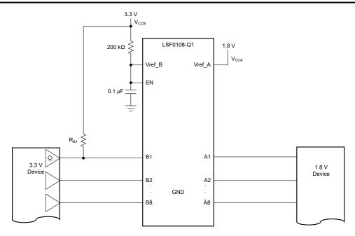
Figure 8-3. Up Translation Example Schematic with Push-Pull and Open Drain Configuration
