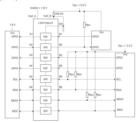
Figure 9-1. Bidirectional Translation to Multiple Voltage Levels
