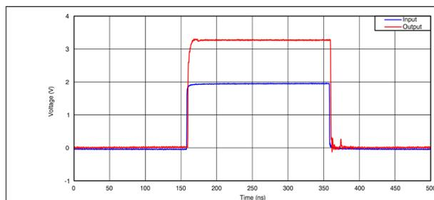
Figure 9-4. Captured Waveform From Above I<sup>2</sup>C Set-Up (1.8 V to 3.3 V at 2.5 MHz)
