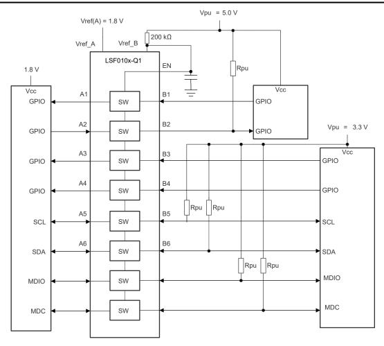
Figure 9-6. Multi-Voltage Translation with the LSF010x-Q1
