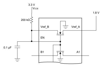
Figure 9-2. Bias Circuitry Inside the LSF010x Device
