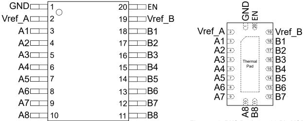
Figure 5-1. PW Package, 20-Pin TSSOP (Transparent Top View)
