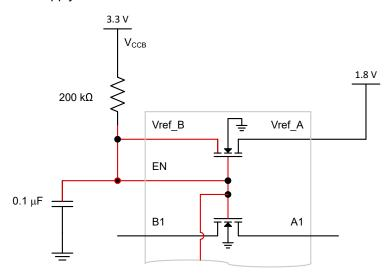
Figure 8-1. EN Pin Tied to V<sub>ref B</sub> Directly and to V<sub>CCB</sub> Through a Pull-Up Resistor
