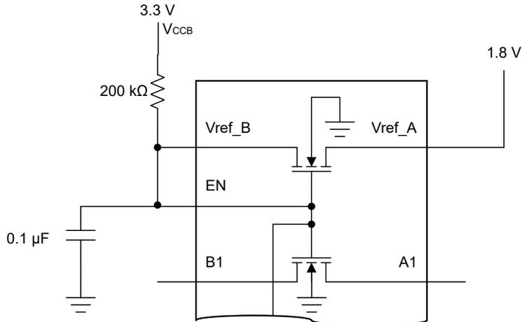
Figure 9-2. Bias Circuitry Inside the LSF010x Device
