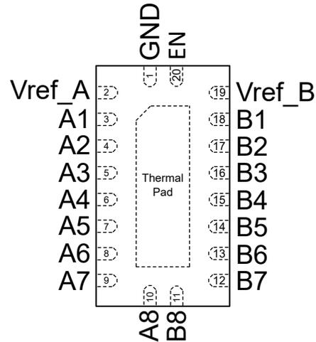
Figure 5-2. RKS Package, 20-Pin VQFN (Transparent Top View)
