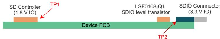
Figure 9-10. Device Placement
