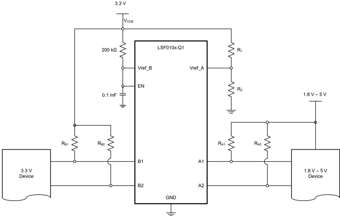
**Figure 9-7. Single Supply Translation with 3.3 V Supply**
