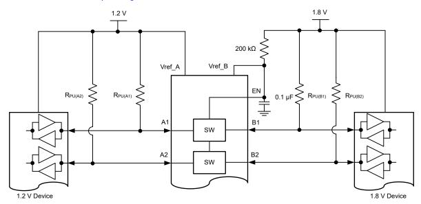
Figure 9-8. 1.2 V to 1.8 V Level Translation with LSF010x-Q1
