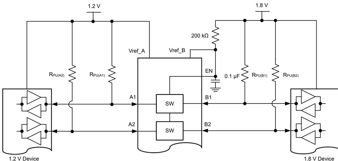
**Figure 9-8. 1.2 V to 1.8 V Level Translation with LSF010x-Q1**
