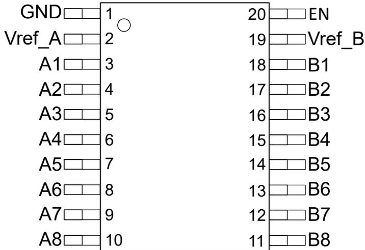
Figure 5-1. PW Package, 20-Pin TSSOP (Transparent Top View)
