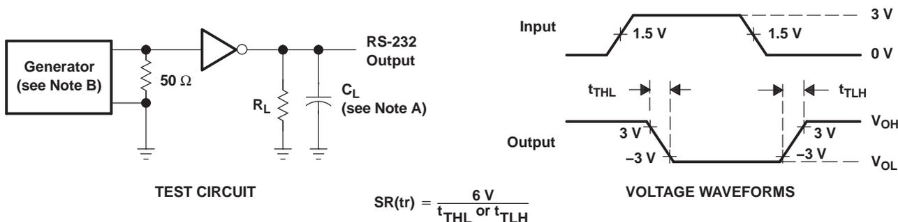
Figure 1. Driver Slew Rate
