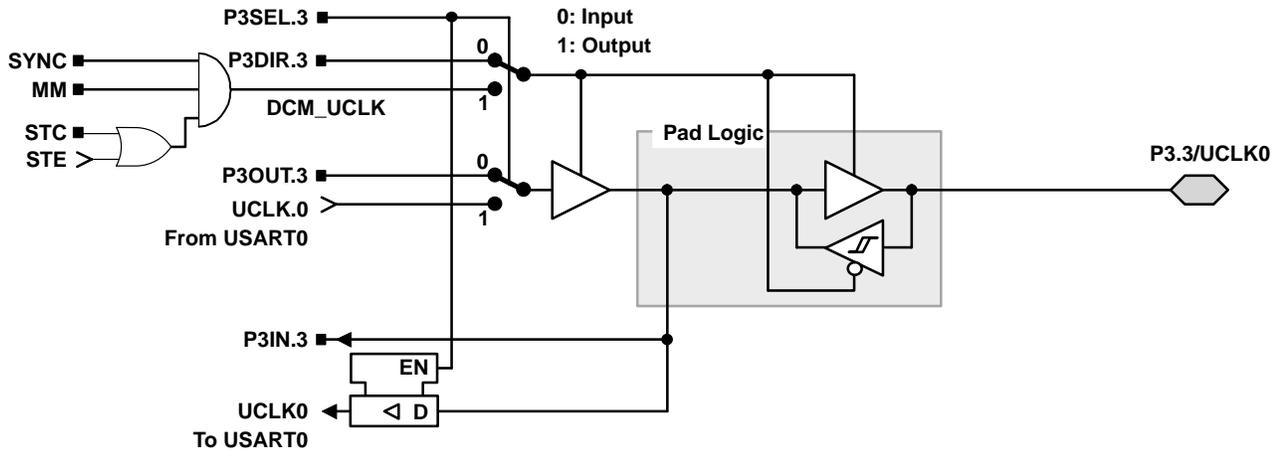
NOTE: UART mode: The UART clock can only be an input. If UART mode and UART function are selected, the P3.3/UCLK0 is always an input.
