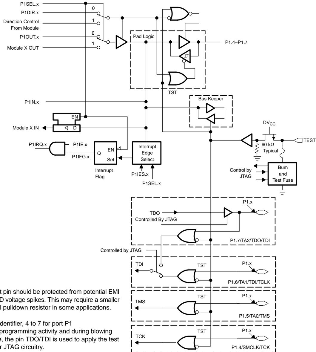
NOTE: The test pin should be protected from potential EMI and ESD voltage spikes. This may require a smaller external pull-down resistor in some applications.
