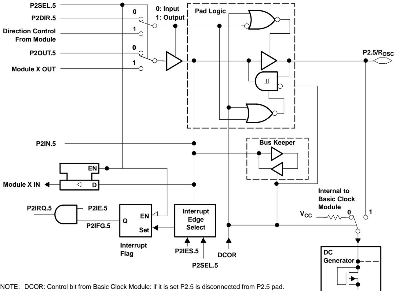
NOTE: DCOR: Control bit from Basic Clock Module: if it is set P2.5 is disconnected from P2.5 pad.
