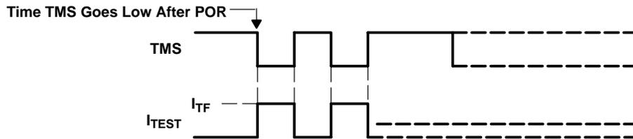
**Figure 10. Fuse Check Mode Current, MSP430F11x2, MSP430F12x2**
