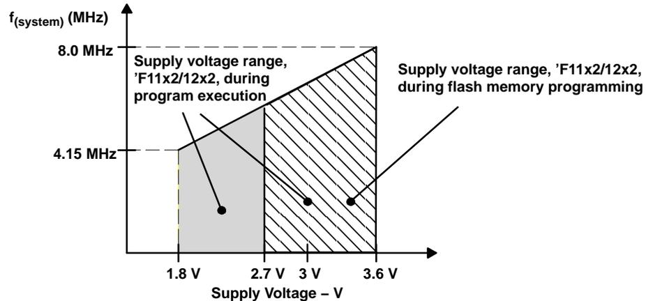
NOTE: Minimum processor frequency is defined by system clock. Flash program or erase operations require a minimum  $V_{CC}$  of 2.7 V.
