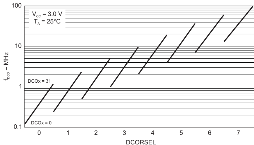
Figure 5-6. Typical DCO Frequency
