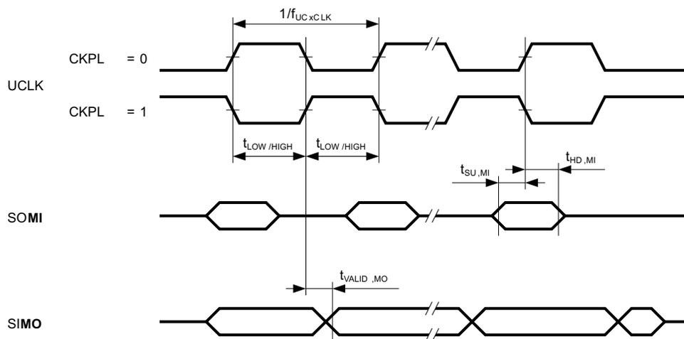
Figure 5-19. SPI Master Mode, CKPH = 1
