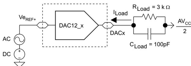
Figure 5-32. Test Conditions for 3-dB Bandwidth Specification
