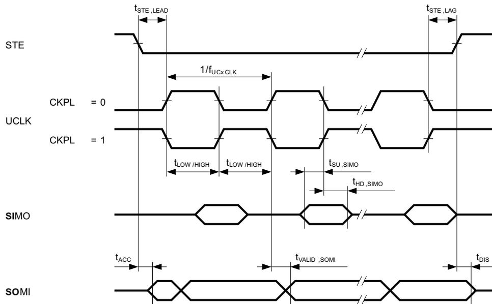
Figure 5-20. SPI Slave Mode, CKPH = 0
