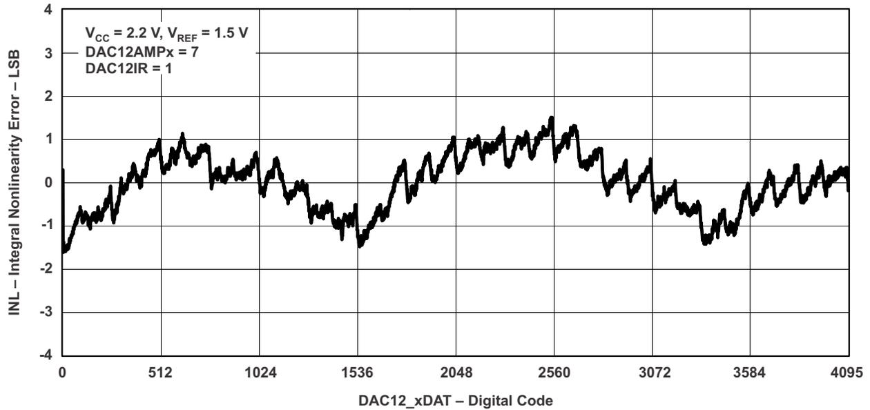
Figure 5-21. Typical INL Error vs Digital Input Data
