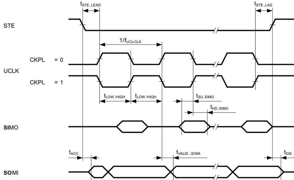
Figure 5-33. SPI Slave Mode, CKPH = 0
