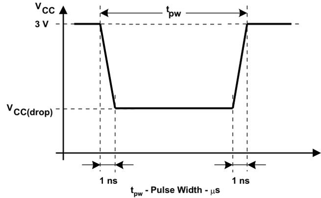
Figure 5-8. V<sub>CC(drop)</sub> Level with a Square Voltage Drop to Generate a POR or BOR Signal
