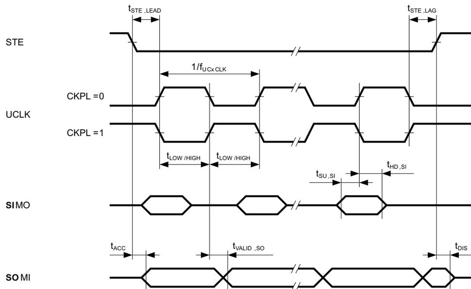
Figure 5-34. SPI Slave Mode, CKPH = 1
