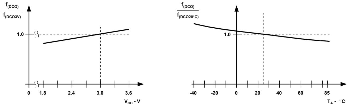
Figure 5-12. DCO Frequency vs Supply Voltage V<sub>CC</sub> and vs Ambient Temperature
