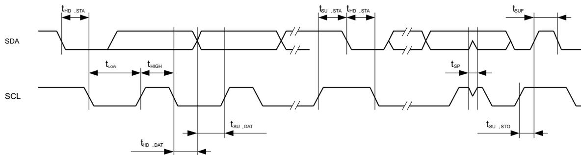
**Figure 5-35. I<sup>2</sup>C Mode Timing**
