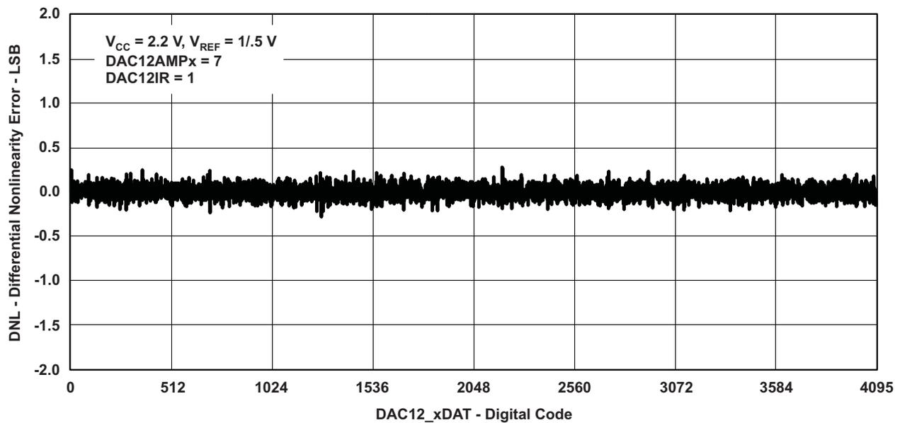
Figure 5-22. Typical DNL Error vs Digital Input Data
