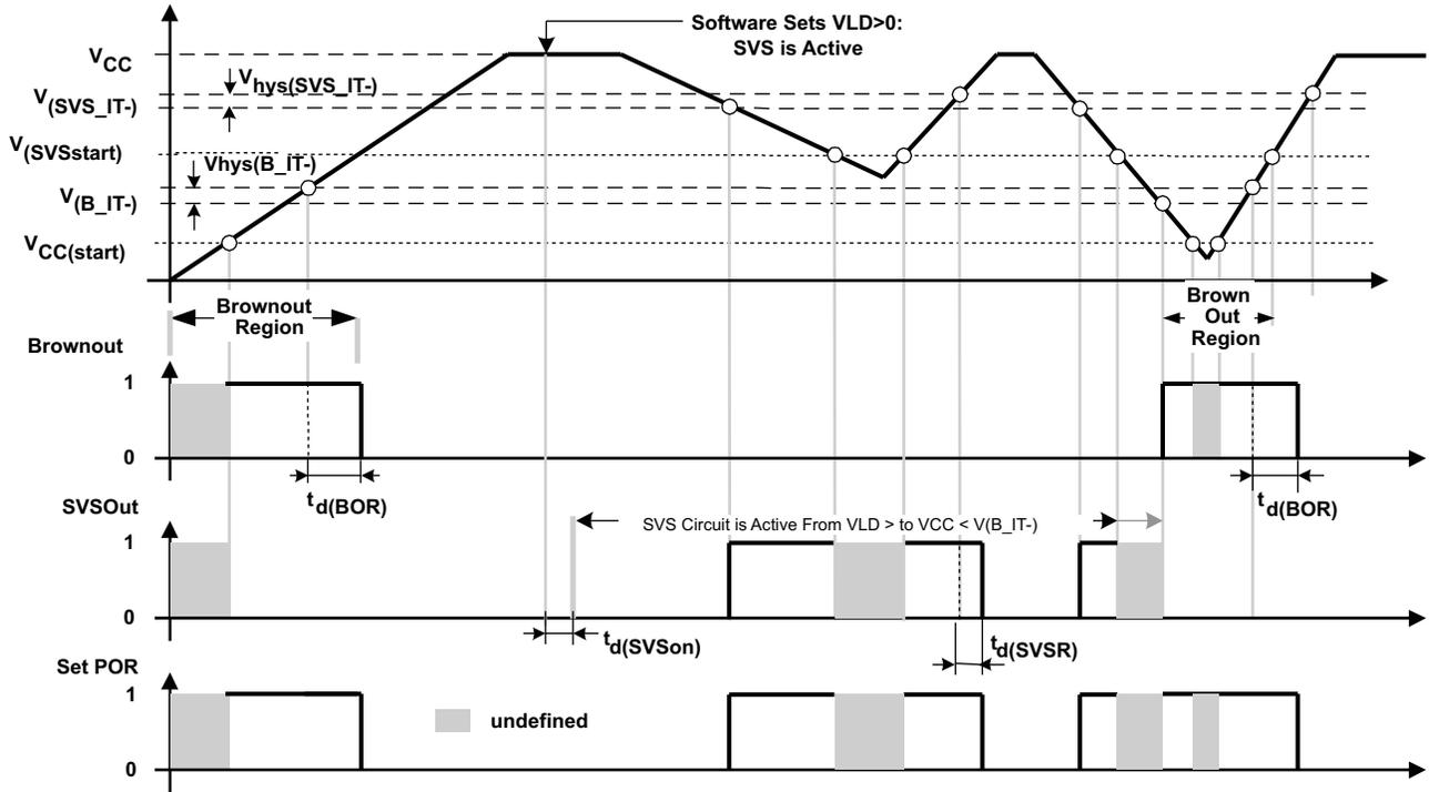
Figure 5-10. SVS Reset (SVSR) vs Supply Voltage
