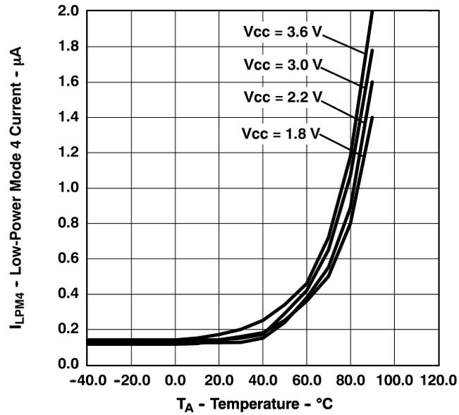
Figure 5-2.  $I_{LPM4}$  – LPM4 Current vs Temperature
