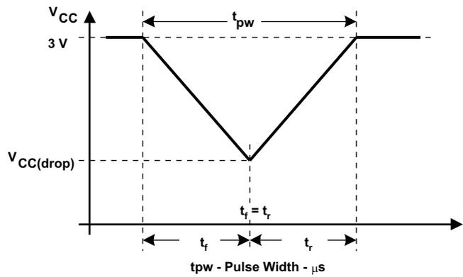
Figure 5-9. V<sub>CC(drop)</sub> Level With a Triangle Voltage Drop to Generate a POR or BOR Signal
