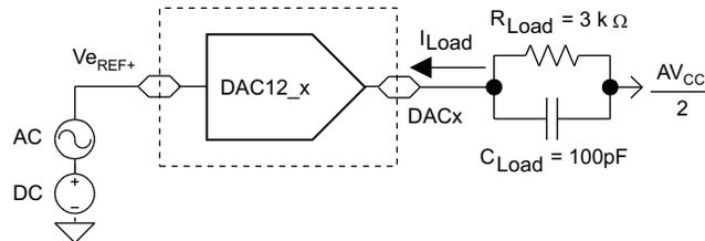
Figure 5-26. Test Conditions for 3-dB Bandwidth Specification
