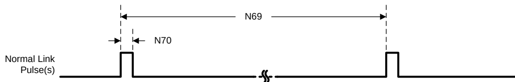
Figure 5-42. 10Base-TX Normal Link Pulse Timing
