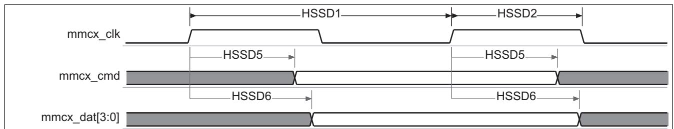
Figure 6-65. MMC/SD/SDIO – High-Speed SD Mode – Data/Command Receive
