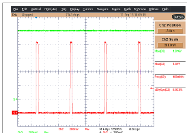
Figure 8-8. Supply Voltage 2.2 V, Peak Signal 1 V
