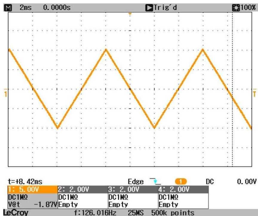
**Figure 31. Full-Scale Output Waveform**
