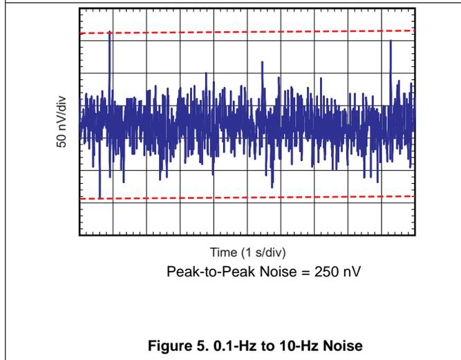
Figure 5. 0.1-Hz to 10-Hz Noise
