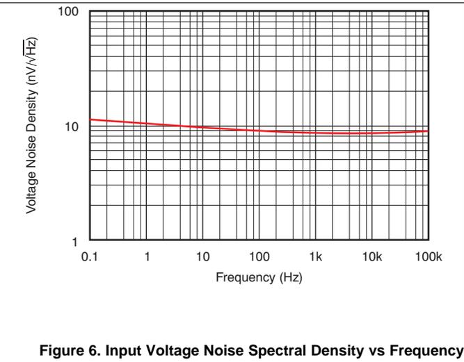
Figure 6. Input Voltage Noise Spectral Density vs Frequency
