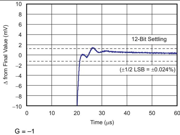
Figure 19. Large-Signal Settling Time (10-V Positive Step)
