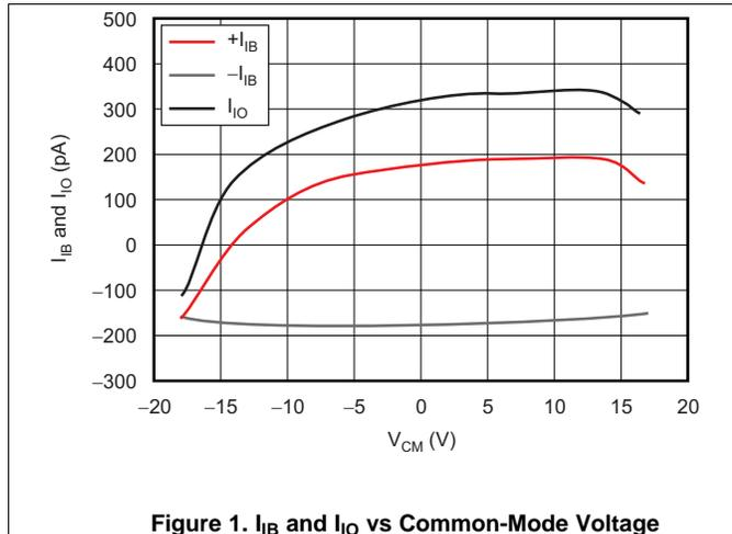
Figure 1.  $I_{IB}$  and  $I_{IO}$  vs Common-Mode Voltage
