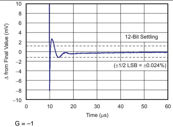
Figure 20. Large-Signal Settling Time (10-V Negative Step)
