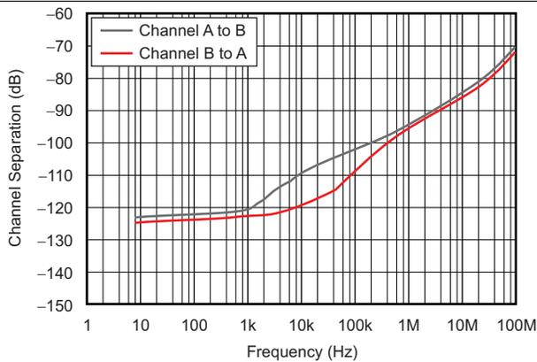
Figure 23. Channel Separation vs Frequency
