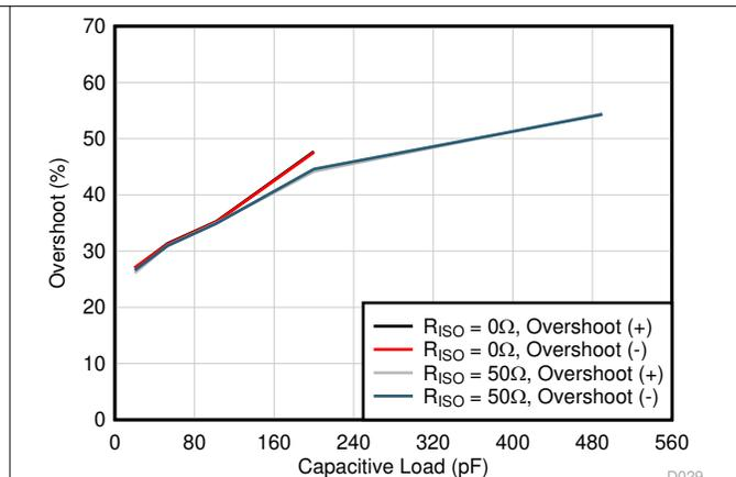
Figure 6-6. Small-Signal Overshoot vs Capacitive Load (20mV<sub>pp</sub> Output Step, G = -1)
