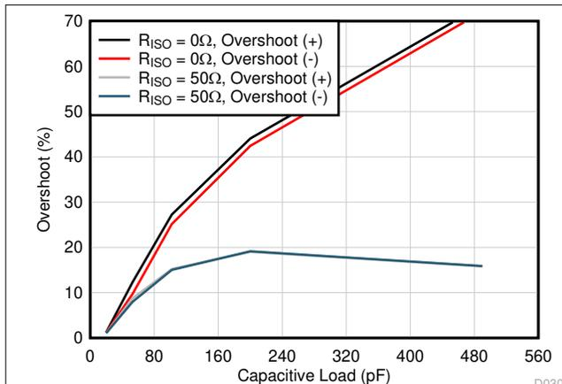
Figure 6-5. Small-Signal Overshoot vs Capacitive Load (20mV<sub>pp</sub> Output Step, G = +1)
