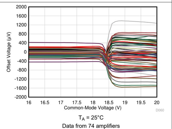
**Figure 5-6. Offset Voltage vs Common-Mode Voltage (Transition Region)**
