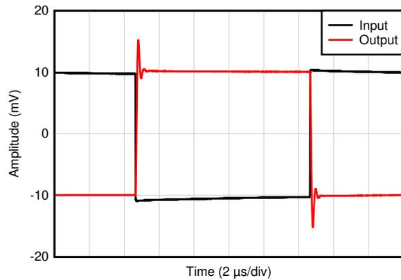
$C_L = 20\text{pF}$ ,  $G = -1$ ,  $20\text{mV}_{pp}$  step response
