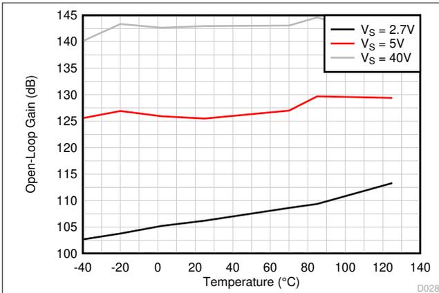
Figure 5-29. Open-Loop Voltage Gain vs Temperature (dB)
