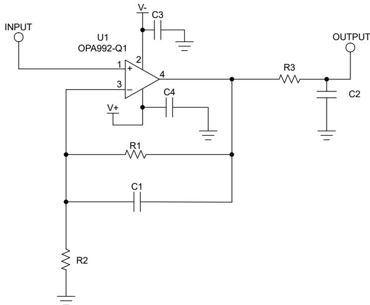
**Figure 7-3. Schematic for Noninverting Configuration Layout Example**
