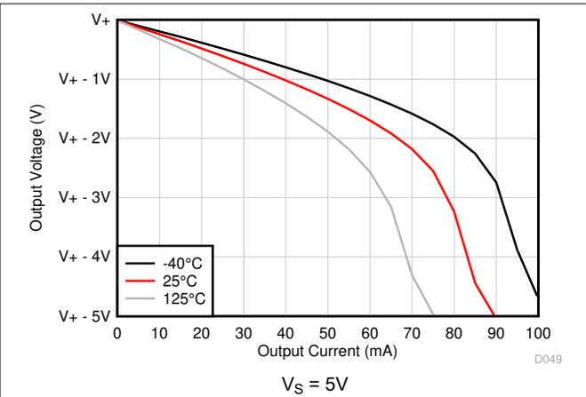
**Figure 5-18. Output Voltage Swing vs Output Current (Sourcing)**
