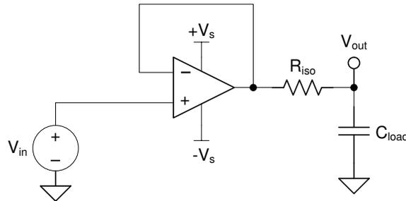
**Figure 6-7. Extending Capacitive Load Drive With the OPA992-Q1**
