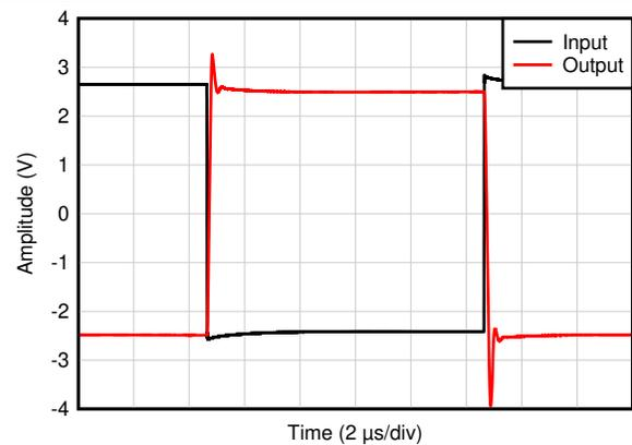
$C_L = 20\text{pF}$ ,  $G = -1$ ,  $5\text{V}_{pp}$  step response
