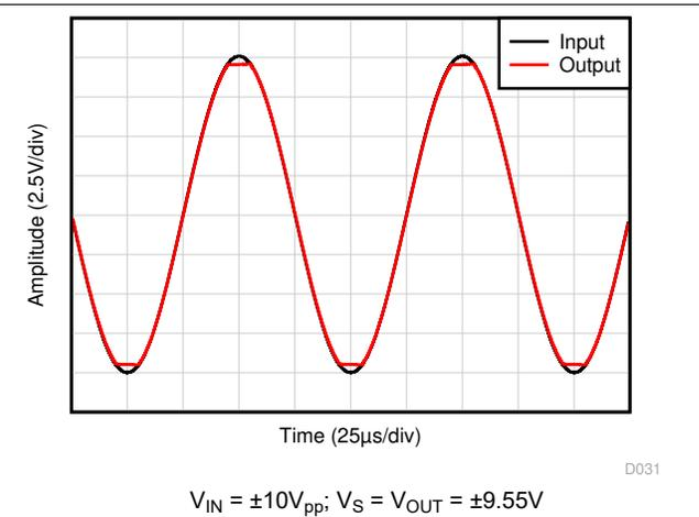
$V_{IN} = \pm 10\text{V}_{pp}$ ;  $V_S = V_{OUT} = \pm 9.55\text{V}$
