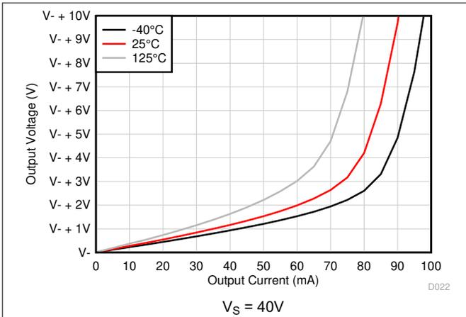
**Figure 5-17. Output Voltage Swing vs Output Current (Sinking)**
