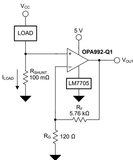
Figure 7-1. OPAx992-Q1 in a Low-Side, Current-Sensing Application
