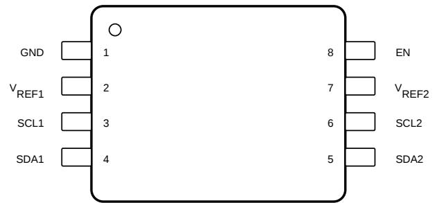
Figure 5-2. DCU Package 8-Pin VSSOP (Top View)
