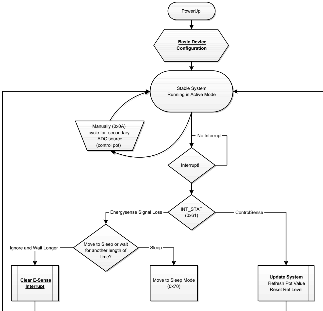
Figure 51. Active Mode Flow Chart
