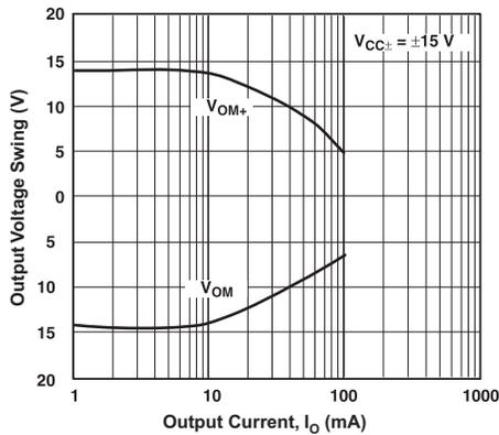
**Figure 5-3. Output Voltage Swing vs Output Current**
