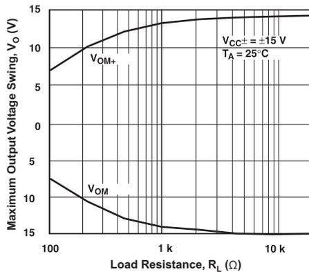
**Figure 5-1. Maximum Output Voltage Swing vs Load Resistance**
