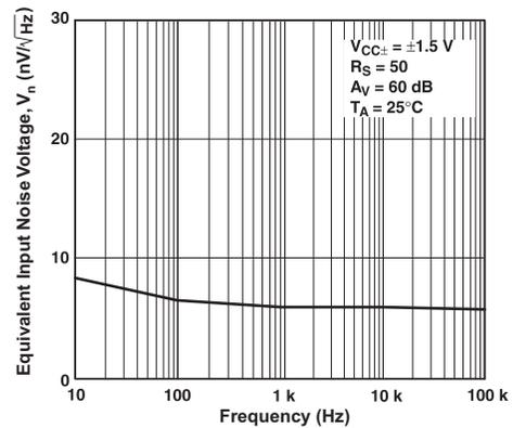
**Figure 5-4. Equivalent Input Noise Voltage vs Frequency**
