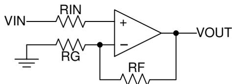
Figure 7-5. Operational Amplifier Schematic for Noninverting Configuration
