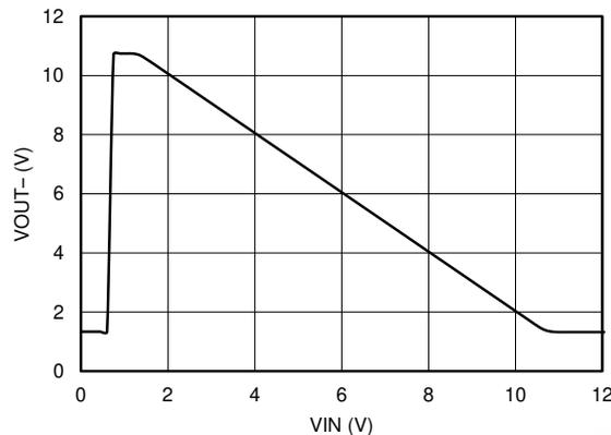
**Figure 7-4. Positive Output Voltage vs Input Voltage**
