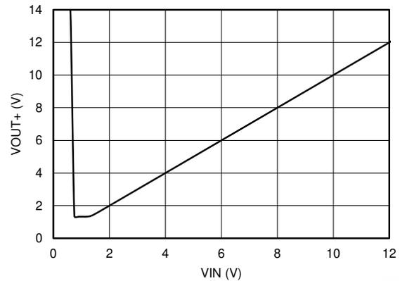
**Figure 7-3. Positive Output Voltage vs Input Voltage**
