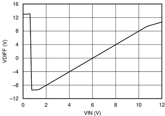
**Figure 7-2. Differential Output Voltage vs Input Voltage**
