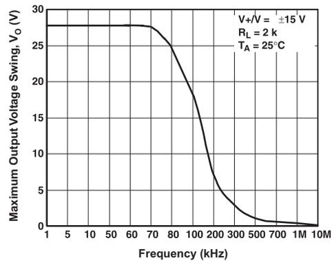
**Figure 5-2. Maximum Output Voltage Swing vs Frequency**
