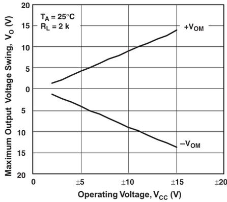
**Figure 5-9. Maximum Output Voltage Swing vs Operating Voltage**
