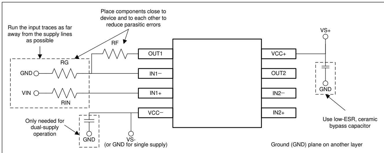
Figure 7-6. Operational Amplifier Board Layout for Noninverting Configuration
