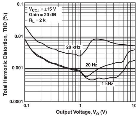
**Figure 5-11. Total Harmonic Distortion vs Output Voltage**
