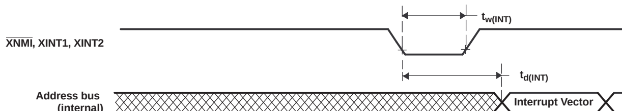
Figure 6-17. External Interrupt Timing
