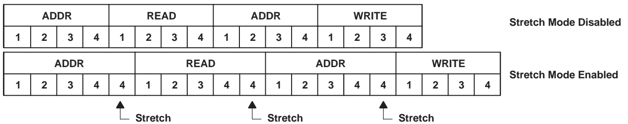
Figure 8. One 32-Bit Nonpage-Mode Read-Write
