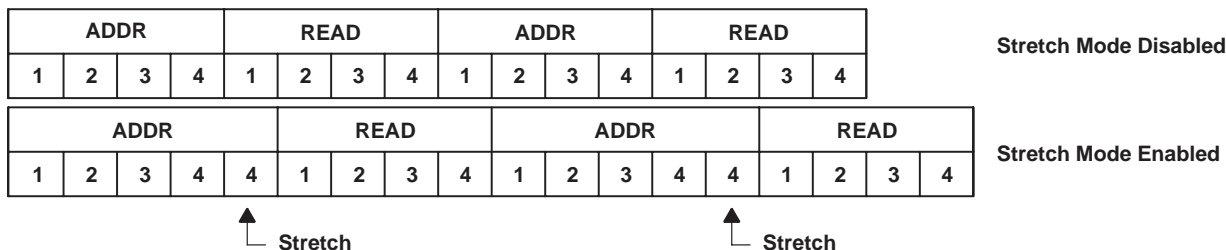
Figure 5. Two 32-Bit Nonpage-Mode Reads
