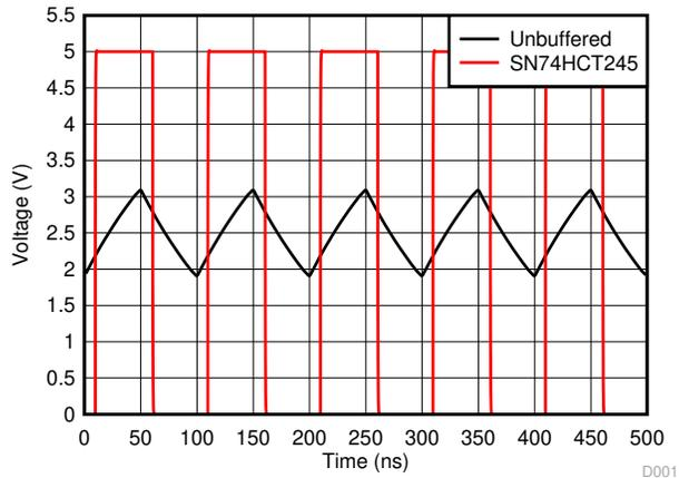
Unbuffered line is directly connected to low current source, SN74HCT245 line is buffered through the transceiver. Both signals are measured at the distant end of the ribbon cable.
