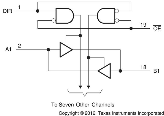
**Figure 8-1. Logic Diagram (Positive Logic)**
