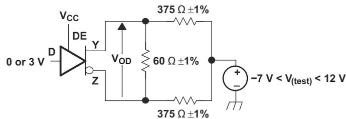
Figure 8-2. Driver  $V_{OD}$  With Common-Mode Loading Test Circuit
