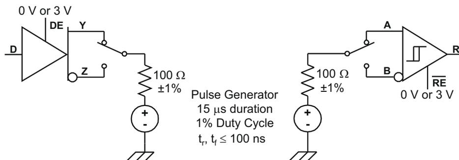
**Figure 8-12. Test Circuit, Transient Overvoltage Test**
