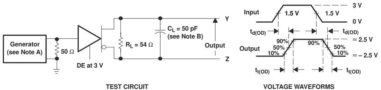
NOTES: A. The input pulse is supplied by a generator having the following characteristics: PRR > 1 MHz, 50% duty cycle,  $t_r \leq 6$  ns,  $t_f \leq 6$  ns,  $Z_O = 50 \Omega$ .
