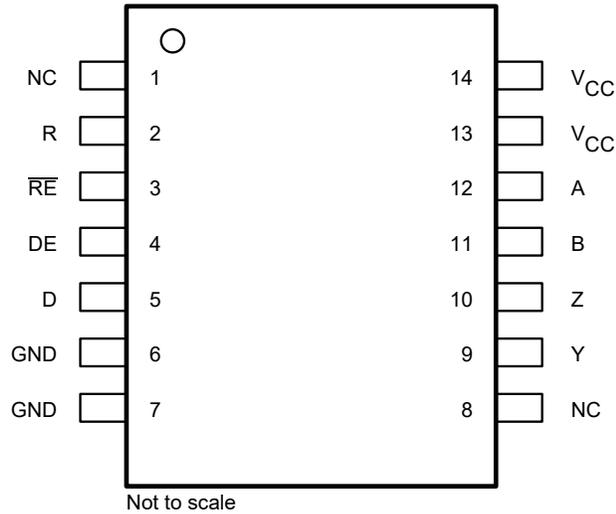
**Figure 5-1. D OR N Package (SOIC)
