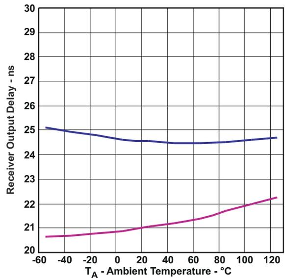
**Figure 6-12. Receiver Propagation DELAY T<sub>I</sub> vs Free-Air Temperature**
