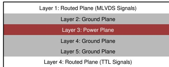
**Figure 11-4. Six-Layer PCB Board**
