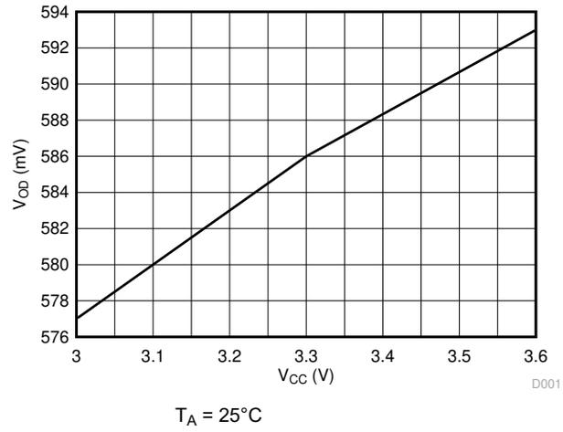
Figure 6-1. Differential Output Voltage vs Supply Voltage
