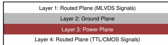
**Figure 11-3. Four-Layer PCB Board**
