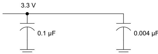
**Figure 9-2. Recommended M-LVDS Bypass Capacitor Layout**
