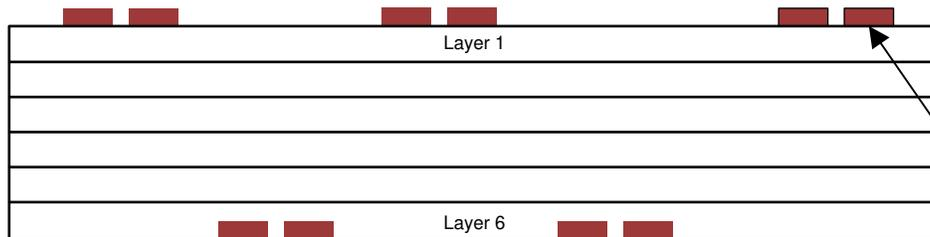
Figure 11-7. Staggered Trace Layout
