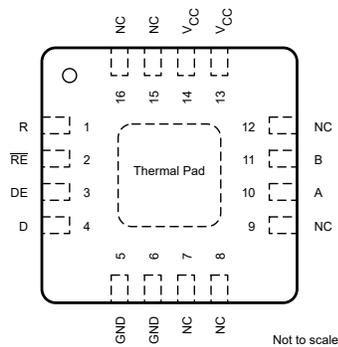
**Figure 5-2. RUM Package 16-Pin WQFN Top View**
