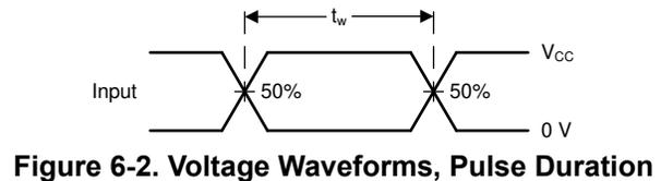
**Figure 6-2. Voltage Waveforms, Pulse Duration**
