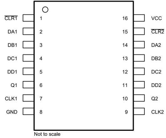
**Figure 4-2. PW Package, 16-Pin TSSOP (Top View)**
