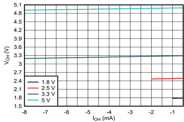
Figure 5-4. Output Voltage vs Current in HIGH State
