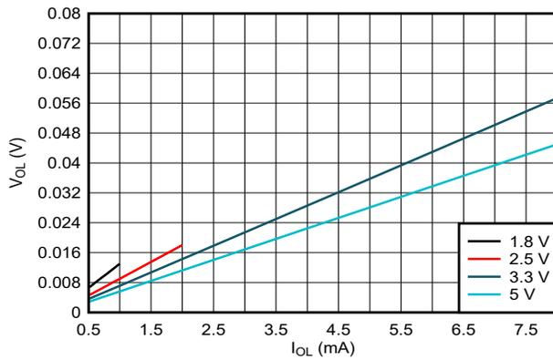
Figure 5-5. Output Voltage vs Current in LOW State
