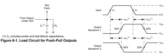
(1) The greater between  $t_{PLH}$  and  $t_{PHL}$  is the same as  $t_{pd}$ .
