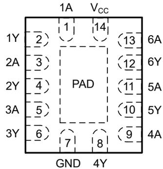
Figure 4-2. BQA Package, 14-Pin WQFN (Top View)
