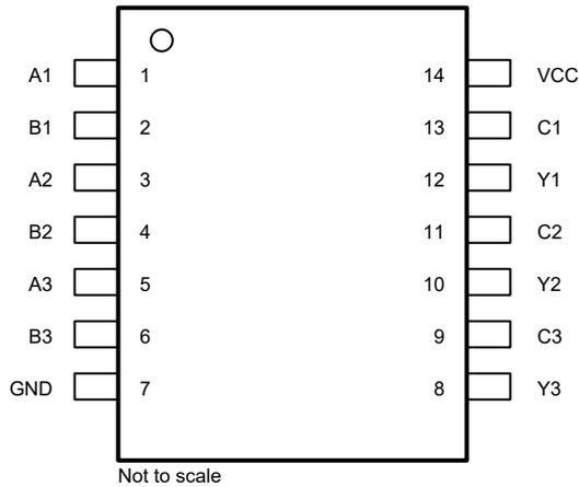
**Figure 4-1. SN74ACT3G97 PW Package, 14-Pin TSSOP (Top View)**
