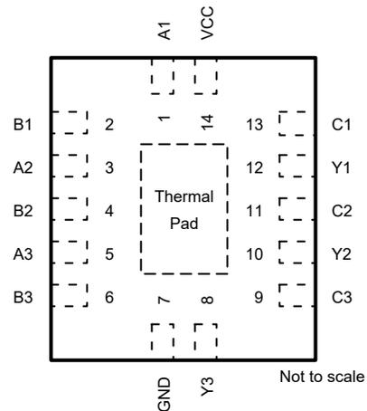
**Figure 4-2. SN74ACT3G97 BQA Package, 14-Pin WQFN (Top View)**
