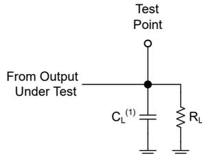
(1)  $C_L$  includes probe and test-fixture capacitance.
