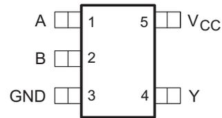
**Figure 4-2. DCK Package 5-Pin SC70 Top View**
