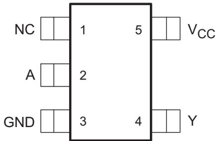
Figure 4-1. DBV Package 5-Pin SOT-23 Top View
