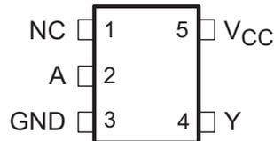
Figure 4-3. DRL Package 5-Pin SOT Top View
