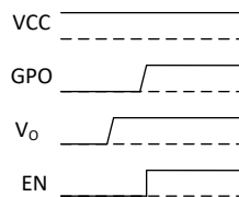
Figure 8-2. Typical Application Timing Diagram
