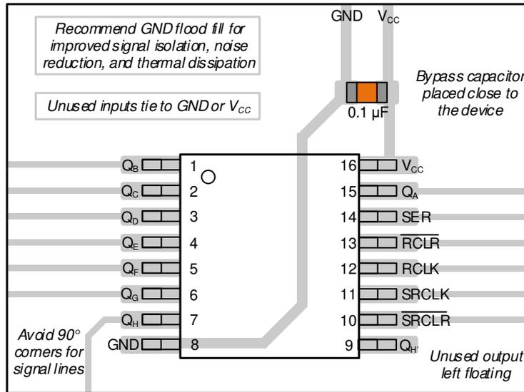
**Figure 8-3. Example Layout for the SN74AHCT594**
