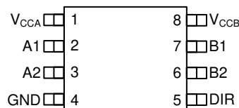
Figure 4-2. DCU Package, 8-Pin VSSOP (Top View)
