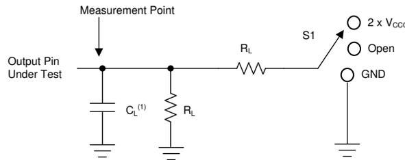
A.  $C_L$  includes probe and jig capacitance.
