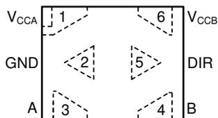
**Figure 5-3. DTQ Package 6-Pin X2SON Transparent Top View**
