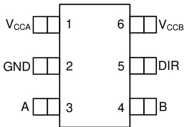
**Figure 5-1. DBV Package 6-Pin SOT-23 Top View**
