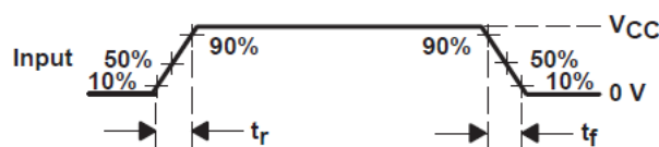
Figure 6-4. Voltage Waveforms Input Rise and Fall Times
