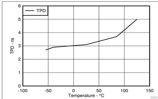
Figure 5-1. TPD Across Temperature at 3.3V  $V_{CC}$
