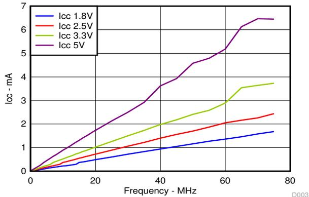
Figure 8-1. I<sub>CC</sub> vs Frequency
