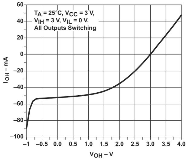
**Figure 5-1. Output Current Drive vs HIGH-level Output Voltage**
