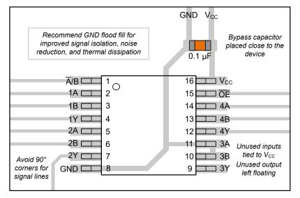
Figure 8-4. Example Layout for the SN74LVC257A
