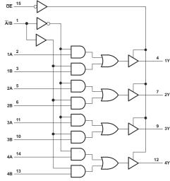
Pin numbers shown are for the D, DB, J, NS, PW, RGY, and W packages. Logic Diagram (Positive Logic)
