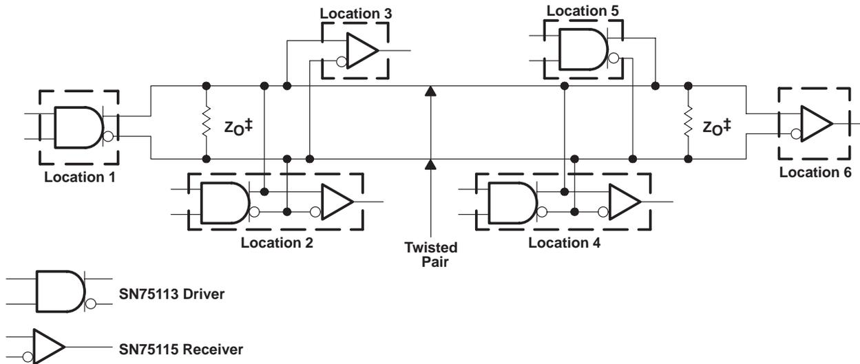
‡  $Z_O = R_T$ . A capacitor may be connected in series with  $Z_O$  to reduce power dissipation.
