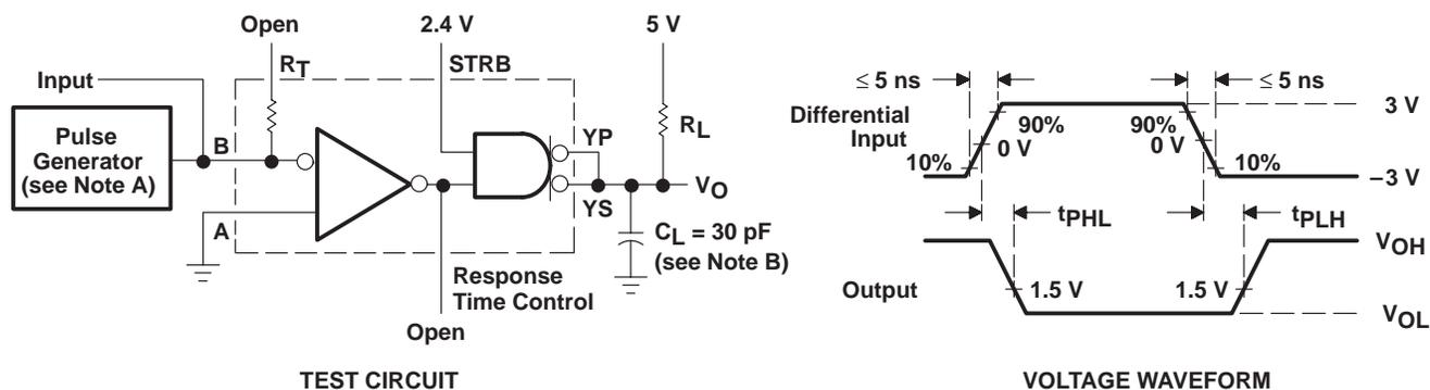
NOTES: A. The pulse generator has the following characteristics:  $Z_O = 50\ \Omega$ ,  $PRR \leq 500\text{ kHz}$ ,  $t_w \leq 100\text{ ns}$ , duty cycle = 50%.
