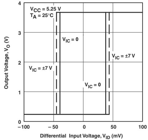
Figure 5-2. Output Voltage vs Differential Input Voltage
