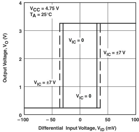
Figure 5-1. Output Voltage vs Differential Input Voltage
