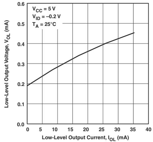
Figure 5-4. Low-Level Output Voltage vs Low-Level Output Current
