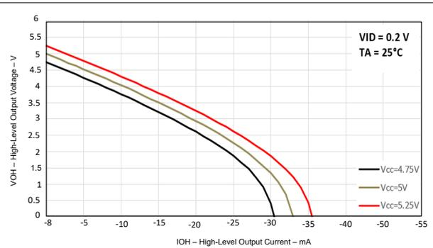
**Figure 5-2. High-level Output Voltage vs High-level Output Current**
