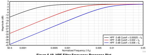
Figure 6-19. HPF Filter Frequency Response Plot
