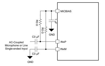
Figure 6-17. AC-Coupled Microphone or Line Single-Ended Input Connection
