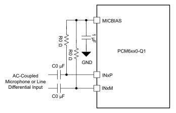
Figure 6-16. AC-Coupled Microphone or Line Differential Input Connection
