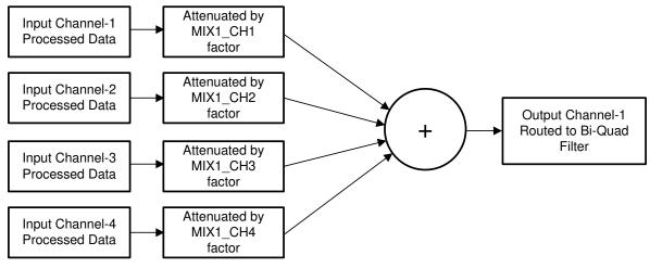
Figure 6-20. Programmable Digital Mixer Block Diagram
