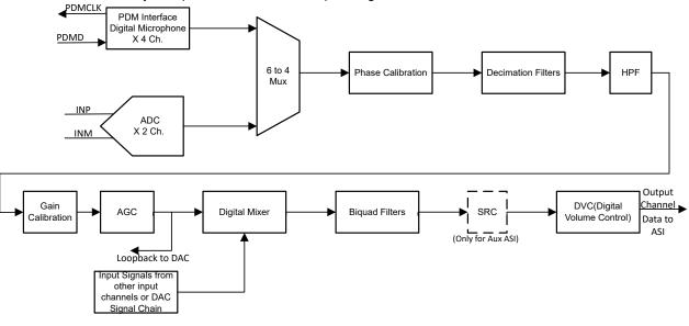
Figure 6-18. ADC Signal-Chain Processing Flowchart
