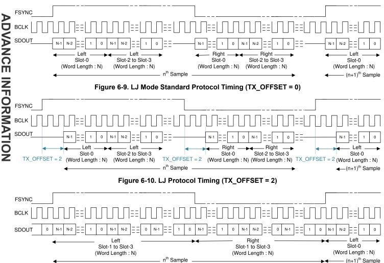
Figure 6-11. LJ Protocol Timing (No Idle BCLK Cycles, TX\_OFFSET = 0)
