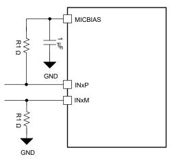
Figure 6-14. DC-Coupled Microphone Differential Input Connection
