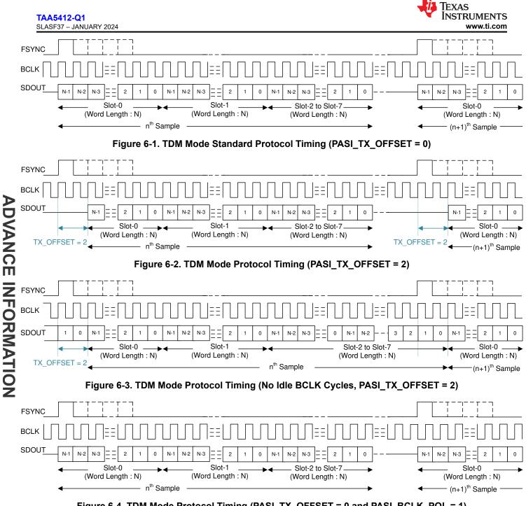
Figure 6-4. TDM Mode Protocol Timing (PASI\_TX\_OFFSET = 0 and PASI\_BCLK\_POL = 1)
