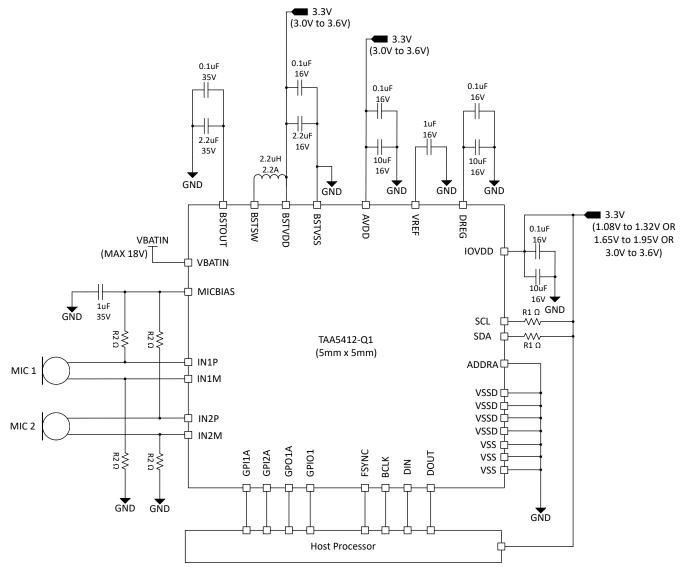
Figure 8-1. Stereo Microphone Block Diagram
