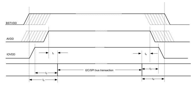
Figure 9-1. Power-Supply Sequencing Requirement Timing Diagram
