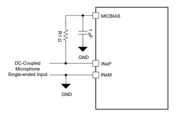
Figure 6-15. DC-Coupled Microphone Single-Ended Input Connection
