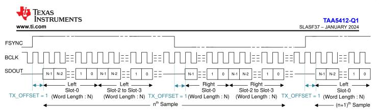
Figure 6-12. LJ Protocol Timing (TX\_OFFSET = 1 and BCLK\_POL = 1)
