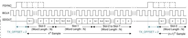
Figure 7-3. TDM Mode Protocol Timing (PASI\_TX\_OFFSET = 2)
