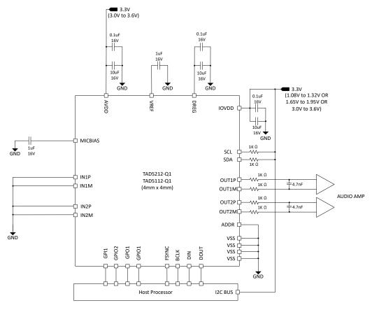
Figure 8-1. Stereo Lineout Block Diagram
