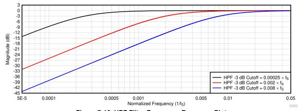
Figure 7-16. HPF Filter Frequency Response Plot
