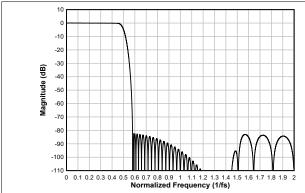
Figure 7-25. Linear Phase Interpolation Filter Magnitude Response
