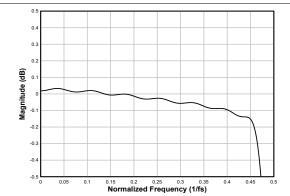
Figure 7-18. Linear Phase Interpolation Filter Pass-Band Ripple
