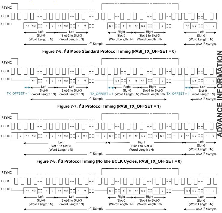
Figure 7-9. I<sup>2</sup>S Protocol Timing (PASI\_TX\_OFFSET = 0 and PASI\_BCLK\_POL = 1)
