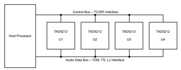
Figure 7-14. Multiple TAD5212 Devices With Shared Control and Audio Data Buses
