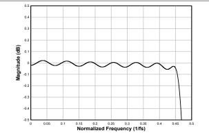
Figure 7-24. Linear Phase Interpolation Filter Pass-Band Ripple
