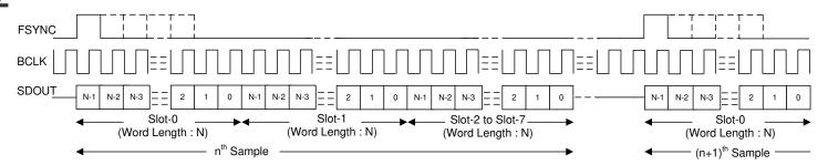
Figure 7-5. TDM Mode Protocol Timing (PASI\_TX\_OFFSET = 0 and PASI\_BCLK\_POL = 1)
