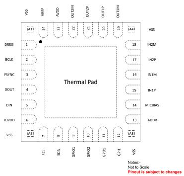
Figure 5-1. 28-Pin QFN With Exposed Thermal Pad, Top View
