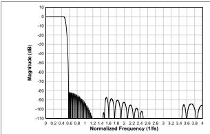
Figure 7-19. Linear Phase Interpolation Filter **Magnitude Response**
