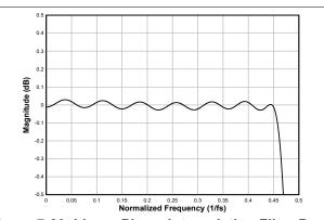
Figure 7-20. Linear Phase Interpolation Filter Pass-**Band Ripple**
