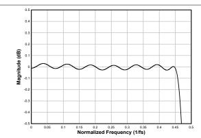
Figure 7-22. Linear Phase Interpolation Filter Pass-Band Ripple
