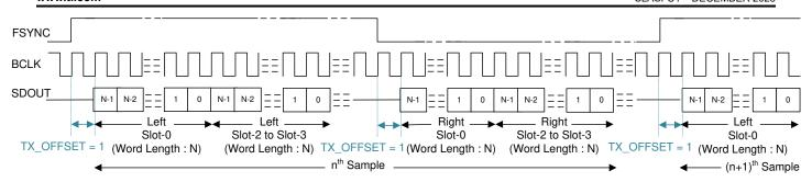
Figure 7-13. LJ Protocol Timing (TX\_OFFSET = 1 and BCLK\_POL = 1)
