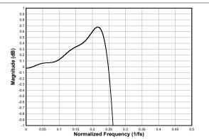
Figure 7-28. Linear Phase Interpolation Filter Pass-Band Ripple
