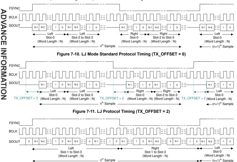
Figure 7-12. LJ Protocol Timing (No Idle BCLK Cycles, TX\_OFFSET = 0)
