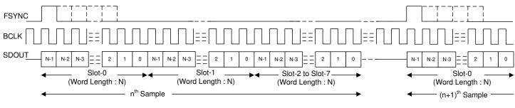
Figure 7-2. TDM Mode Standard Protocol Timing (PASI TX OFFSET = 0)
