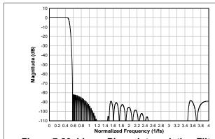
Figure 7-23. Linear Phase Interpolation Filter Magnitude Response
