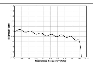
Figure 7-26. Linear Phase Interpolation Filter Pass-Band Ripple
