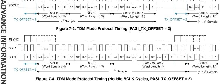
Figure 7-4. TDM Mode Protocol Timing (No Idle BCLK Cycles, PASI TX OFFSET = 2)
