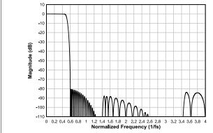
Figure 7-17. Linear Phase Interpolation Filter Magnitude Response
