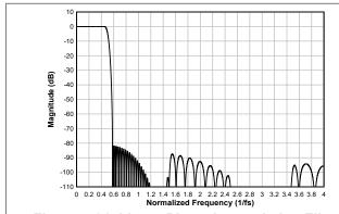
Figure 7-21. Linear Phase Interpolation Filter Magnitude Response
