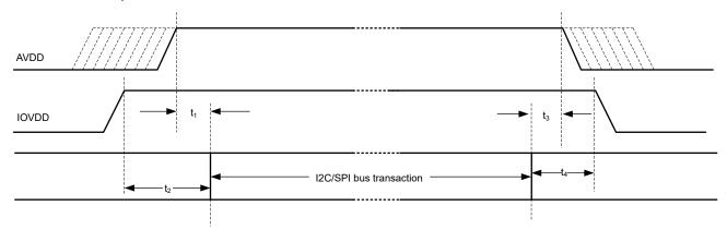
Figure 9-1. Power-Supply Sequencing Requirement Timing Diagram
