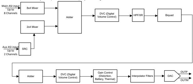
Figure 7-15. DAC Signal-Chain Processing Flowchart
