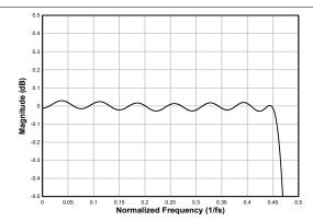
Figure 8-10. Linear Phase Interpolation Filter Pass-Band Ripple
