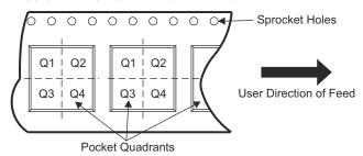
Reel Width W1 Reel Package Pin1 Package A0 В0 K0 Р1 w Pins SPQ Device Diamete Drawing (mm) Quadrant Type (mm) (mm) (mm) (mm) (mm) (mm) XTAD5242IRGER VQFN RGE 24 3000 330.0 12.4 4.25 4.25 1.15 8.0 12.0 Q1
