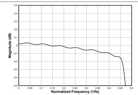
Figure 8-8. Linear Phase Interpolation Filter Pass-Band Ripple
