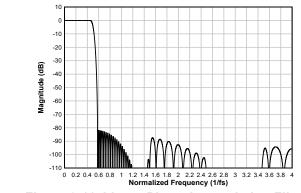
Figure 8-11. Linear Phase Interpolation Filter Magnitude Response
