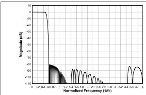
Figure 8-7. Linear Phase Interpolation Filter Magnitude Response
