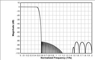
Figure 8-15. Linear Phase Interpolation Filter Magnitude Response
