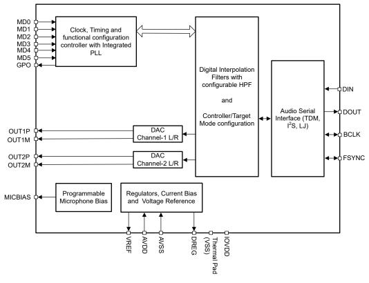
Figure 8-1. Functional Block Diagram
