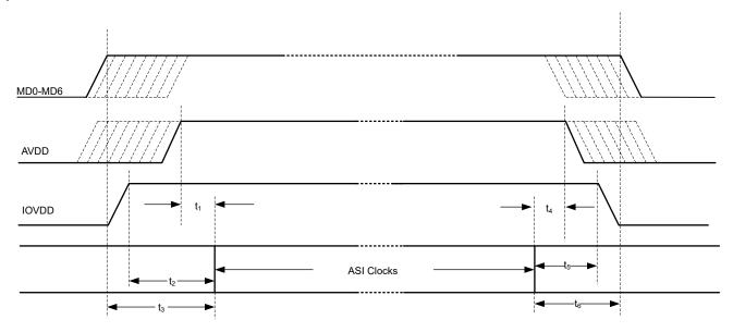
Figure 10-1. Power-Supply Sequencing Requirement Timing Diagram
