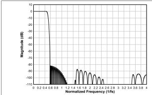
Figure 8-9. Linear Phase Interpolation Filter Magnitude Response
