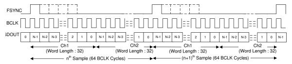
Figure 8-3. TDM Mode Protocol Timing (MD0 shorted to AVDD with 4.7K Ohms) In Controller Mode
