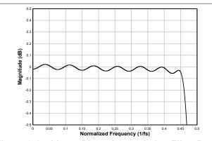
Figure 8-14. Linear Phase Interpolation Filter Pass-Band Ripple
