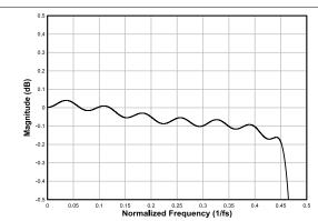
Figure 8-16. Linear Phase Interpolation Filter Pass-Band Ripple
