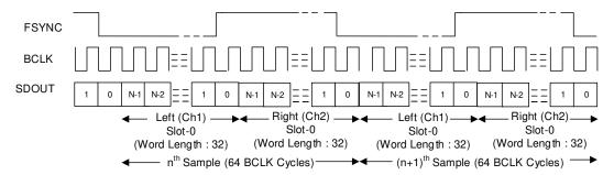
Figure 8-5. I<sup>2</sup>S Protocol Timing (MD0 shorted to AVDD) In Controller Mode
