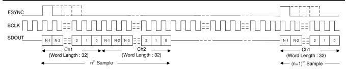
Figure 8-2. TDM Mode Protocol Timing (MD0 shorted to ground with 4.7K Ohms) In Target Mode
