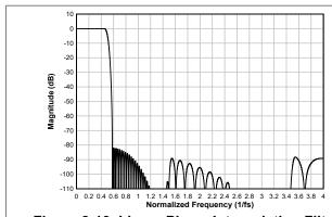
Figure 8-13. Linear Phase Interpolation Filter Magnitude Response
