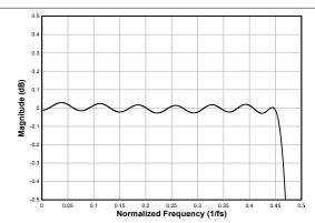
Figure 8-12. Linear Phase Interpolation Filter Pass-Band Ripple
