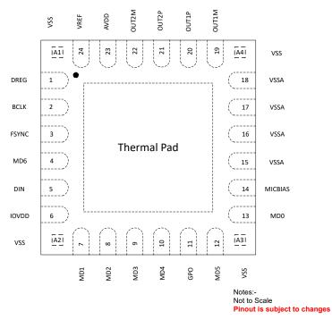
Figure 5-1. TAD5242 Pinout
