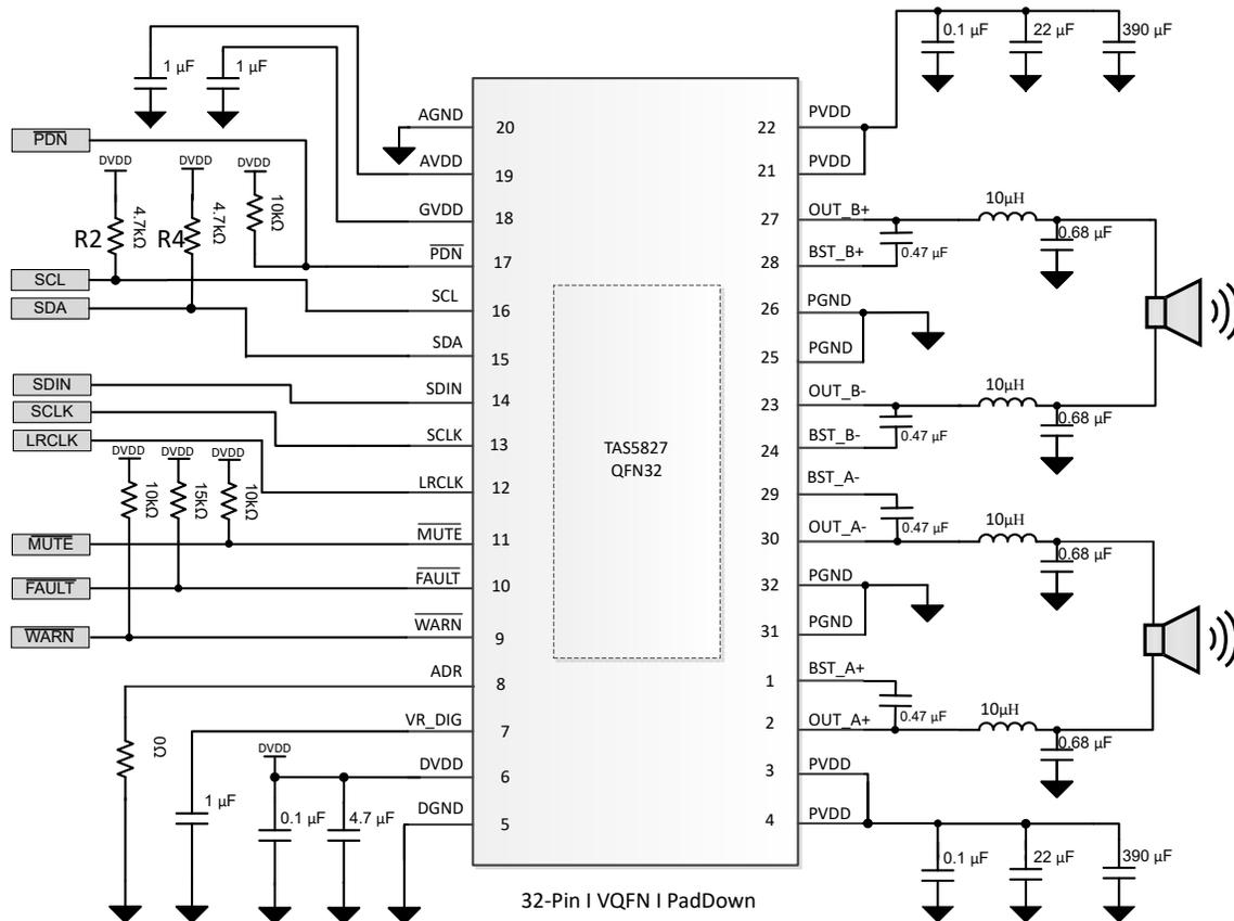
Figure 8-1. 2.0 (Stereo BTL) System Application Schematic
