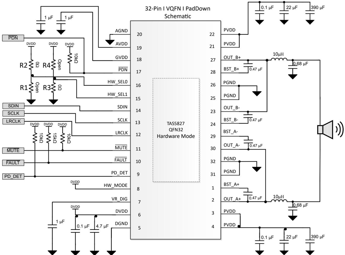
Figure 6-11. Typical Hardware Control Mode Application Schematic-PBTL Mode
