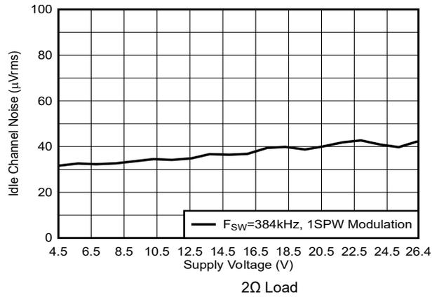
**Figure 5-68. Idle Channel Noise vs Supply Voltage**
