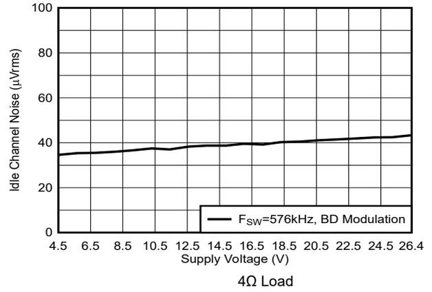
**Figure 5-52. Idle Channel Noise vs Supply Voltage**
