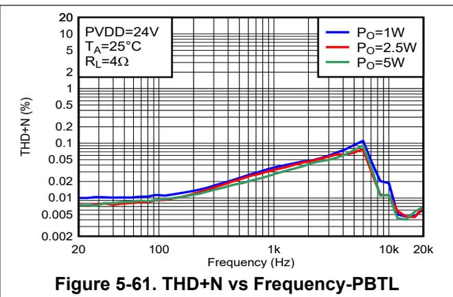
Figure 5-61. THD+N vs Frequency-PBTL
