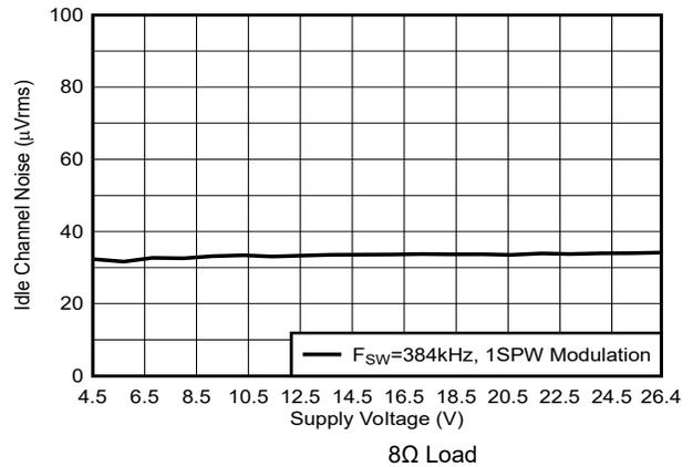
Figure 5-33. Idle Channel Noise vs Supply Voltage
