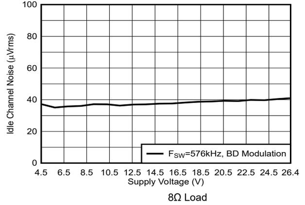
**Figure 5-14. Idle Channel Noise vs Supply Voltage**
