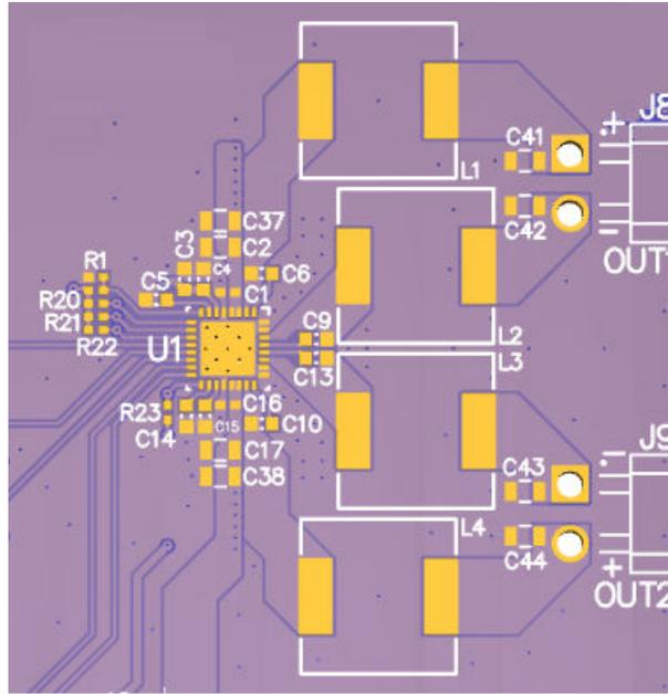
**Figure 8-4. 2.0 (Stereo BTL) Top Copper View**
