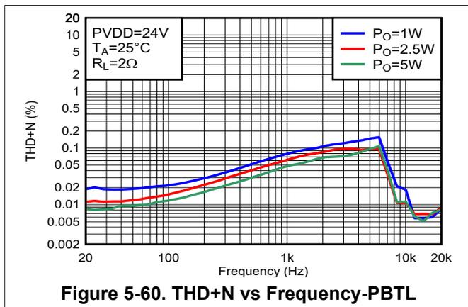
Figure 5-60. THD+N vs Frequency-PBTL
