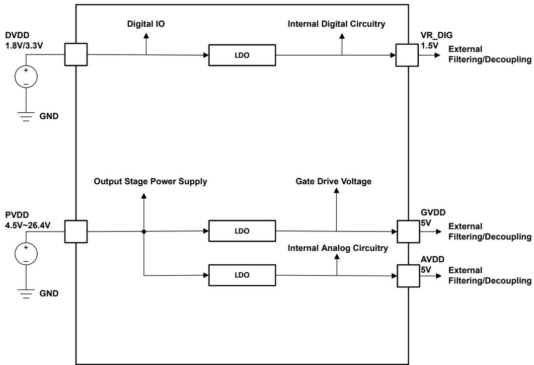
**Figure 8-5. Power Supply Functional Block Diagram**
