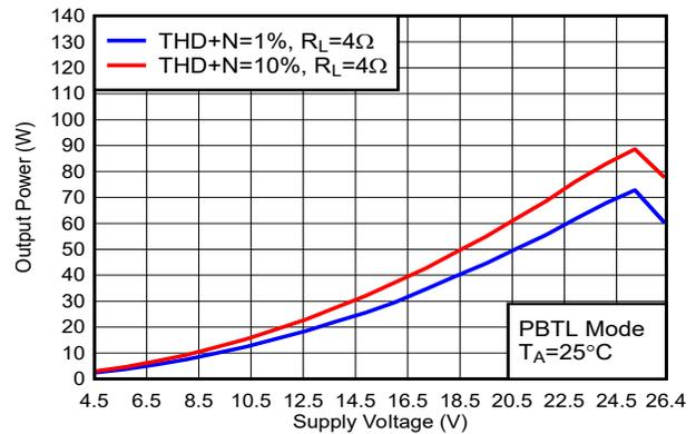
Figure 5-67. Output Power vs Supply Voltage
