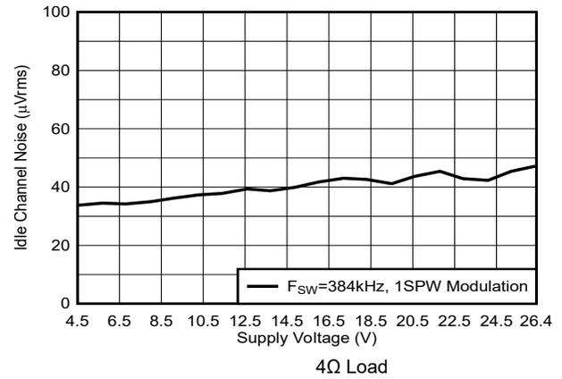
**Figure 5-69. Idle Channel Noise vs Supply Voltage**
