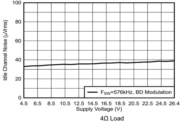
**Figure 5-13. Idle Channel Noise vs Supply Voltage**
