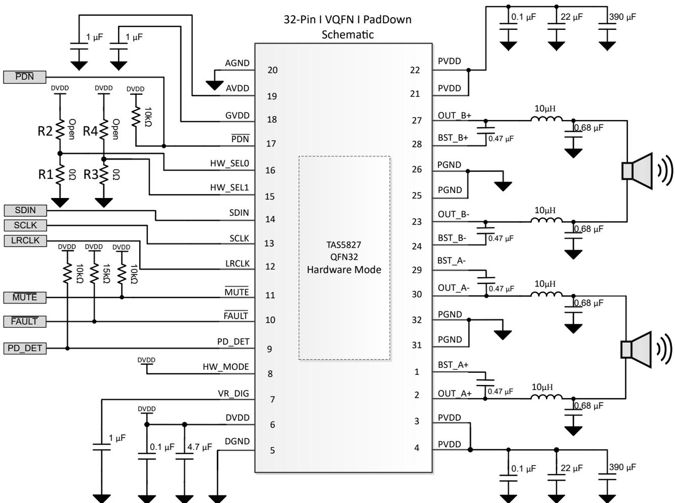
**Figure 6-10. Typical Hardware Control Mode Application Schematic-BTL Mode**
