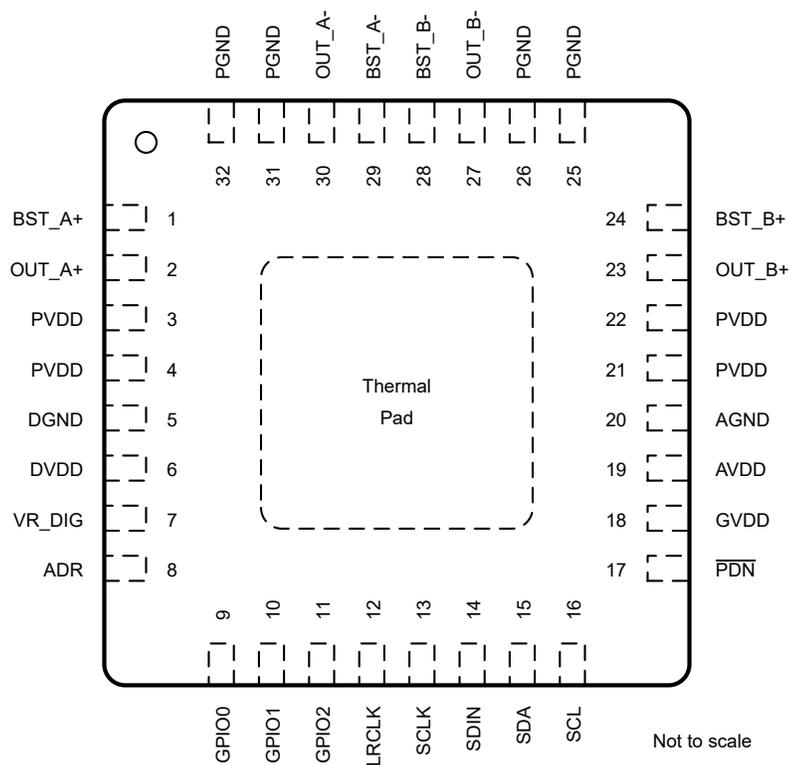
**Figure 4-1. RHB (VQFN) Package, 32-Pin PadDown, Software Mode, Top View**
