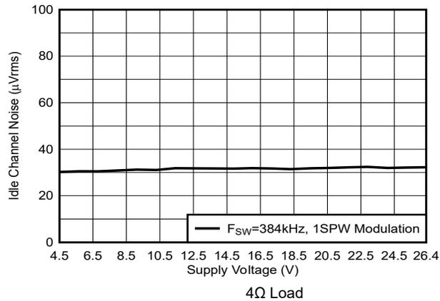
Figure 5-32. Idle Channel Noise vs Supply Voltage
