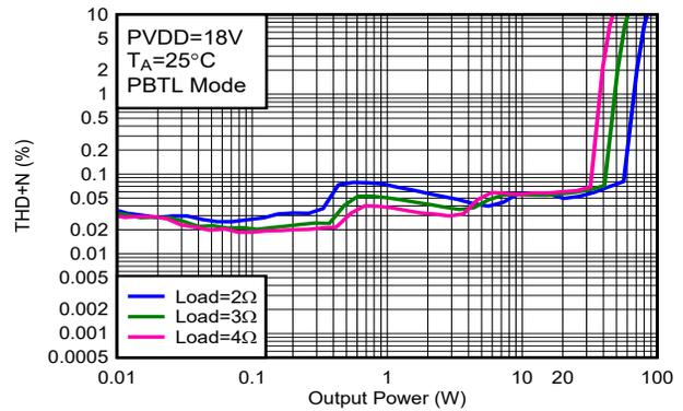
Figure 5-63. THD+N vs Output Power-PBTL
