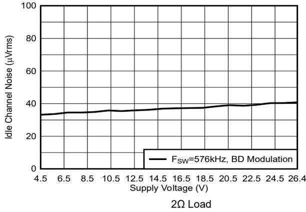
**Figure 5-51. Idle Channel Noise vs Supply Voltage**
