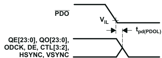
Figure 8-8. Delay From \overline{PDO} Low to Hi-Z Outputs
