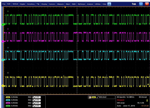
THVD2410 V_{CC} = 5\text{ V} R_L = 50\ \Omega Random (PRBS7) data at 500 kbps
