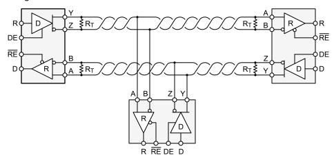
Figure 8-1. Typical RS-485 Network With Half-Duplex Transceivers
