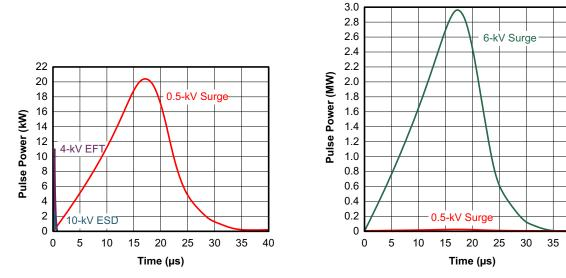
Figure 8-4. Power Comparison of ESD, EFT, and Surge Transients
