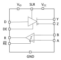
Figure 7-1. THVD9491-SEP Block Diagram
