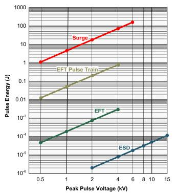
Figure 8-5. Comparison of Transient Energies
