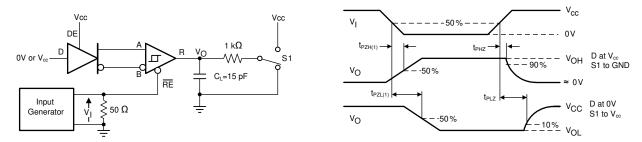
Figure 6-7. Measurement of Receiver Enable/Disable Times With Driver Enabled
