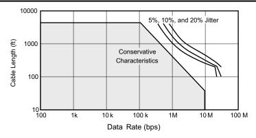
Figure 8-2. Cable Length vs Data Rate Characteristic
