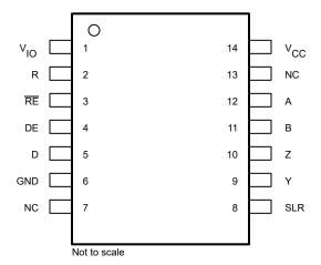
Figure 4-1. D (SOIC) Package 14-Pin (Top View)
