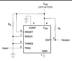
Figure 6-2. Circuit for Monostable Operation
