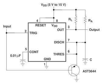
Figure 7-1. Circuit for Missing-Pulse Detector
