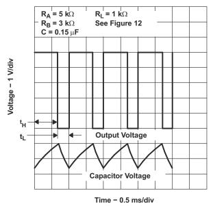
Figure 6-6. Typical Astable Waveforms
