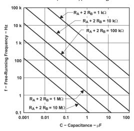
Figure 6-8. Free-Running Frequency
