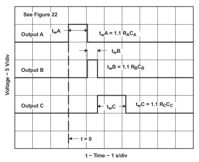
Figure 7-8. Sequential Timer Waveforms
