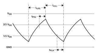
Figure 6-7. Trigger and Threshold Voltage Waveform
