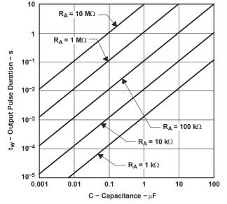
Figure 6-4. Output Pulse Duration vs Capacitance
