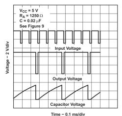
Figure 6-9. Divide-by-Three Circuit Waveforms
