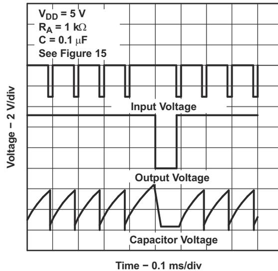
Figure 7-2. Completed Timing Waveforms for Missing-Pulse Detector
