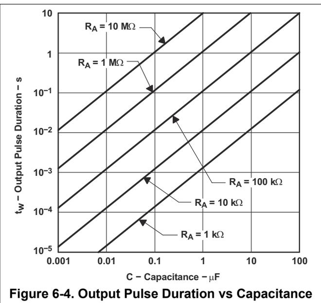
**Figure 6-4. Output Pulse Duration vs Capacitance**
