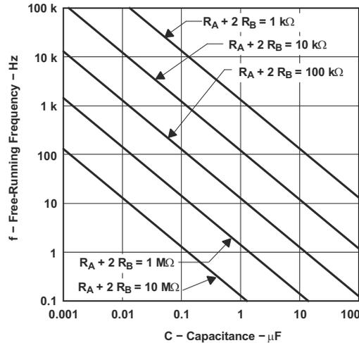
**Figure 6-8. Free-Running Frequency**
