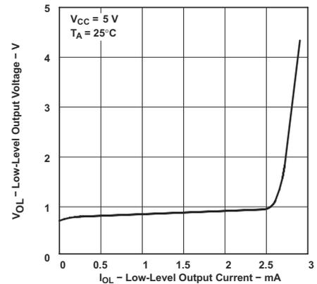
Figure 6-18. Low-Level Output Voltage vs Low-Level Output Current
