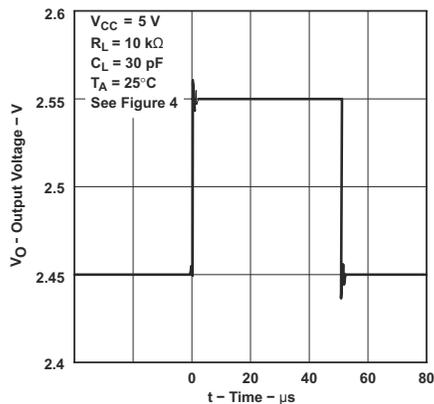
Figure 6-35. Voltage-Follower Small-Signal Pulse Response
