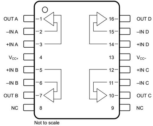
**Figure 5-4. TLE2024: DW Package, 16-Pin (Top View)**
