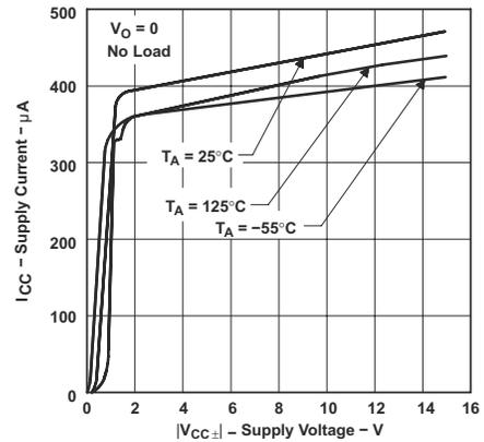
Figure 6-28. TLE2022 Supply Current vs Supply Voltage
