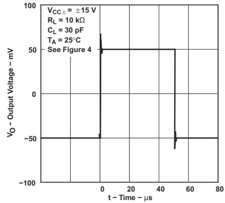
Figure 6-34. Voltage-Follower Small-Signal Pulse Response
