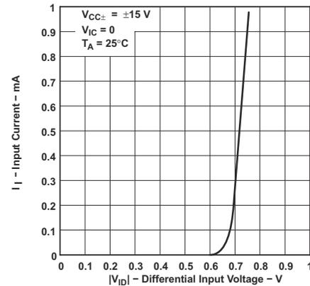
Figure 6-10. Input Current vs Differential Input Voltage
