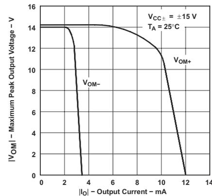
Figure 6-12. TLE2022 Maximum Peak Output Voltage vs Output Current
