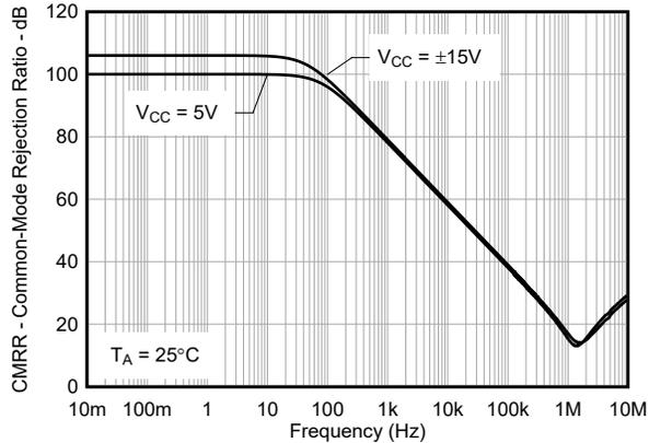
Figure 6-33. TLE202x Common-Mode Rejection Ratio vs Frequency
