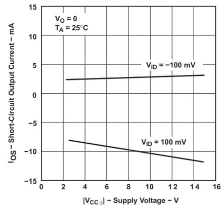
Figure 6-24. TLE2022 and TLE2024 Short-Circuit Output Current vs Supply Voltage
