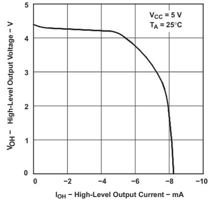
Figure 6-16. TLE2022 and TLE2024 High-Level Output Voltage vs High-Level Output Current
